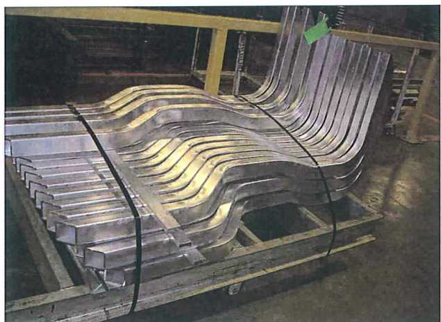
Figure 11. Package of fabricated Club Car XRT 1550 frame members ready for shipment.
