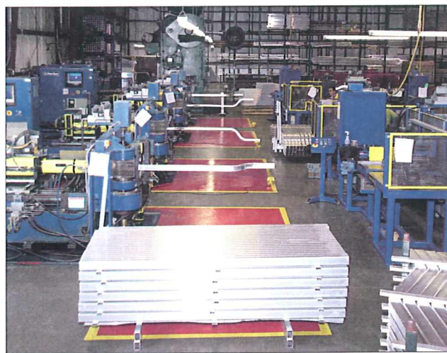
Figure 4. Load of side rails ready for bending operations.
