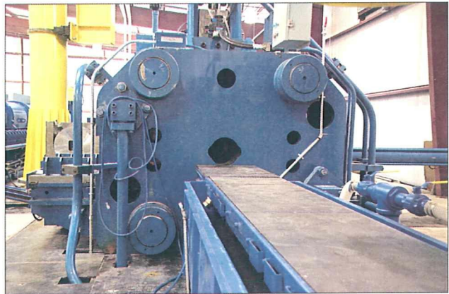
Figure 9. The R.L. Best press will handle 8" billets.
